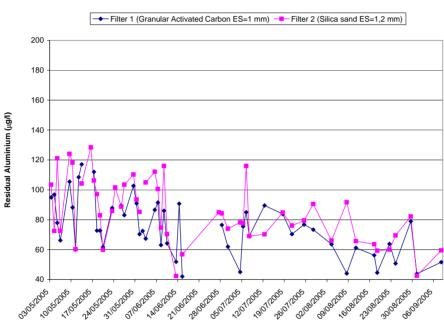
ALUMINUM IN FILTER EFFLUENT
