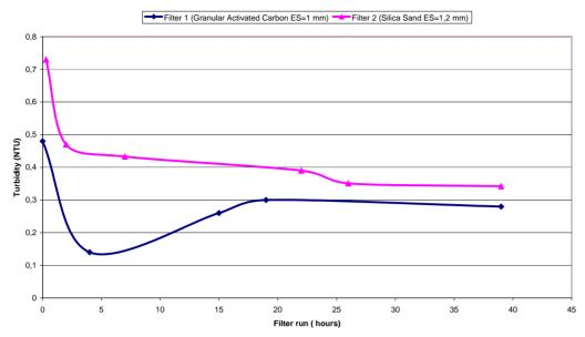
Chart 3: Turbidity at the filter effluent
