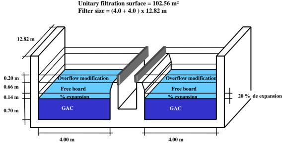
Figure 1: Schematic design modification of the GAC filter
