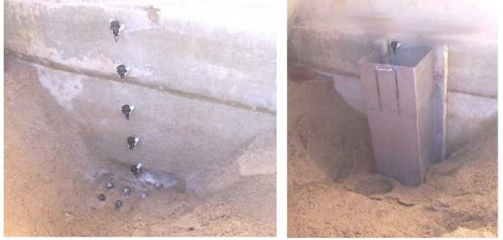
Photography 1: Pressure drop measurement devices and protection
